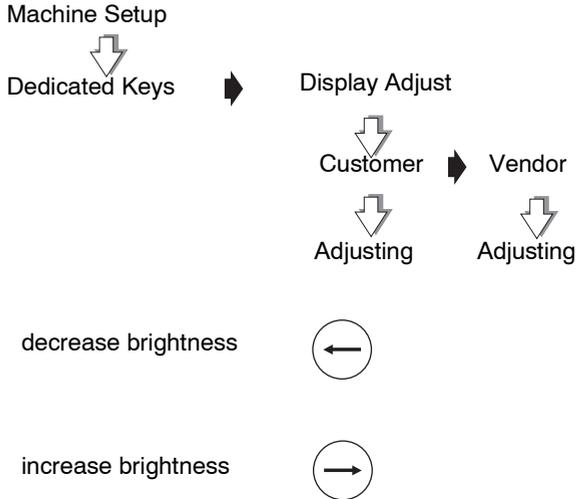
**Figure 5.9 Adjusting display brightness**
