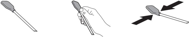
Hold swab between thumb and forefinger and snap at position indicated..
