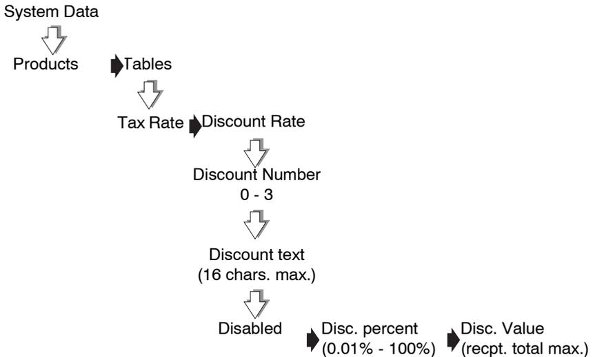
**Figure 3.6 Programming a fixed discount**
